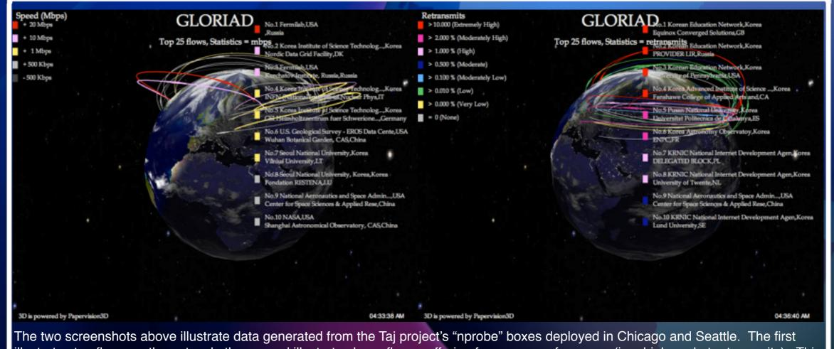
The two screenshots above illustrate data generated from the Taj project's "nprobe" boxes deployed in Chicago and Seattle. The first illustrates top flows on the network; the second illustrates large flows suffering from poor performance (i.e., high packet retransmits). This data was formerly generated from GLORIAD's packeteer system (limited to 1 Gbps circuit capacity).
